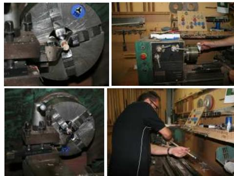
Zeljko expertly removes a Brass Ferrule & replaces it with a Black Nylon Ferrule
